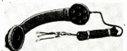
Appearance of the new "Universal" French hand-set, comprising special mike and high resistance, light-weight receiver. (No. 225.)
